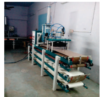
CHAPATI COOLANT CONVEYOR
